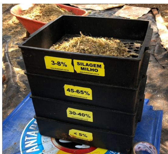
Figure 1 – Penn State Particle Separator.
