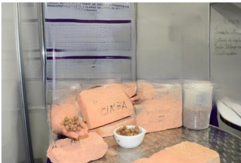
Figure 5 – Reuse of açaí seeds as an energy source in brick production.
