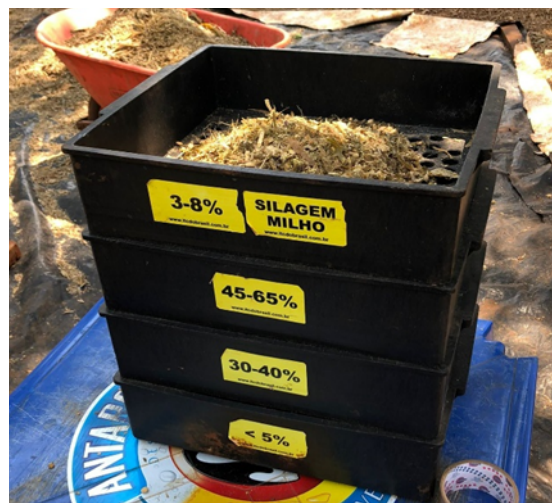
Figure 1 - Penn State Particle Separator.
