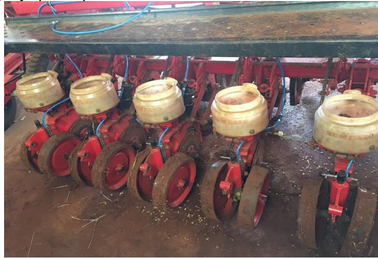
Figure 2. Equipment used for the application of biostimulants in the sowing furrow. The blue hose refers to spray tips coupled to the seeder.
