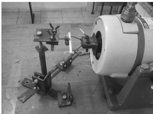
**Figure 4.** Fixation of the coffee fruit-stem system sample during the trials performed to analyze the effect of the impact of a rigid rod over the fruits.
