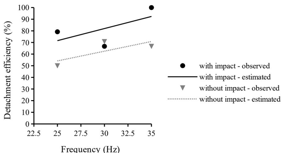
**Figure 9.** Effect of the mechanical vibrations transmission, with or without impact, over the detachment efficiency of the coffee fruits.
