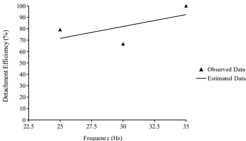
**Figure 5.** Effect of the frequency of vibration over the detachment efficiency of the coffee fruits obtained from the Trial 2 (mechanical vibrations transmitted to the coffee fruit-stem system due the impact of a rigid rod).
