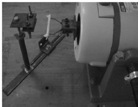
Figure 3. Representation of the two configurations of the vibration trials and its respectively fixation structures: (A) structure mounted on the mobile base of the shaker used on vibration trials without impact and (B) static structure for samples fixation and structure used for fixation of the rigid rod used on vibration trials performed by using impact over the coffee fruits.
