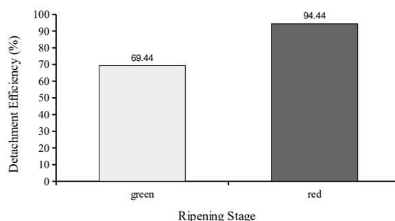
**Figure 6.** Effect of the ripening stage over the detachment efficiency of the coffee fruits obtained from the Trial 2 (mechanical vibrations transmitted to the coffee fruit-stem system due the impact of a rigid rod).
