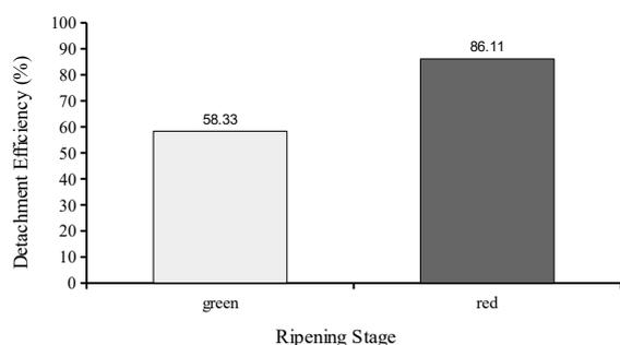
**Figure 7.** Effect of the ripening stage over the detachment efficiency of the coffee fruits obtained from the Trial 3 (mechanical vibrations transmitted with or without impact of a rigid rod on the coffee fruit-stem system).
